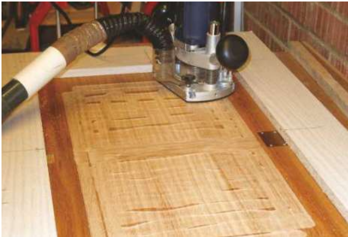
▲ Pic.23 Make sure that the jig is securely attached when routing the flap
